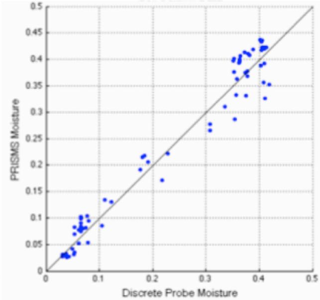
**Plots above show the strong correlation of PRISMS to reference methods in laboratory soil column and soil trough tests.**
