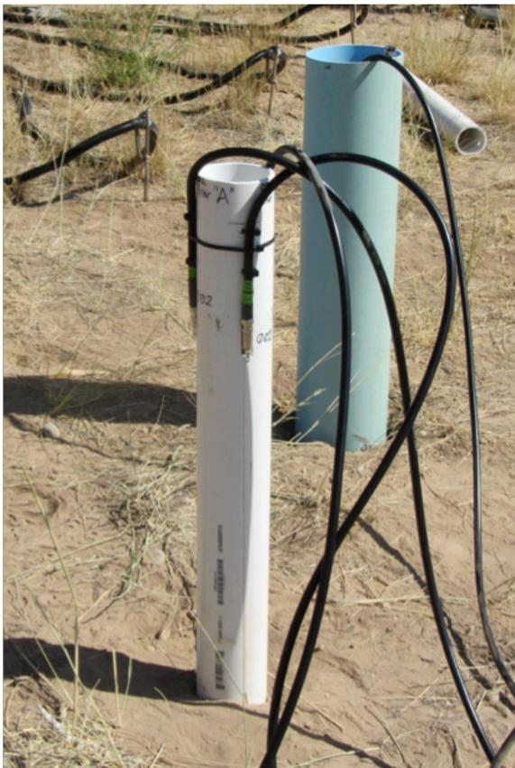
**PRISMS sensor element on the outside of a rigid borehole liner.**
